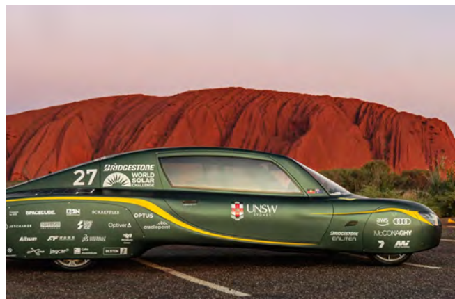
SUNSWIFT RACING SUNSWIFT 7 | AUSTRALIA NO. 11 Sunswift has competed in the Bridgestone World Solar Challenge (BWSC) 12 times and has been part of the Cruiser Class since its inception. Their latest vehicle, Sunswift 7, prioritises efficiency through holistic optimisation across mechanical, electrical, and solar systems. With a drag coefficient of 0.095 and rolling resistance of 0.1, the car delivers impressive mechanical performance while maintaining a focus on roadworthiness and practicality. The BWSC offers Sunswift a platform to demonstrate its technological advancements and test innovations aimed at progressing electric vehicle development. As an Australian team, Sunswift values the chance to engage with international engineering students and share in the collaborative spirit of the event.
