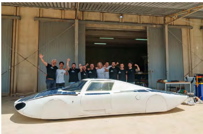
ARCHIMEDE THALIA | ITALY NO. 24 Archimede is a newly formed team making its debut at the Bridgestone World Solar Challenge. In just over a year, they've developed a solar car that blends sustainability, innovation, and performance. Covered in high-efficiency solar panels and built with lightweight materials like carbon fibre and aluminium, the car is designed for both competition and future scalability. For Archimede, the BWSC is a testbed for their engineering solutions and a key step in their growth as a startup. The team looks forward to the challenge of the Outback and the chance to share their vision for a cleaner, solar-powered future.
