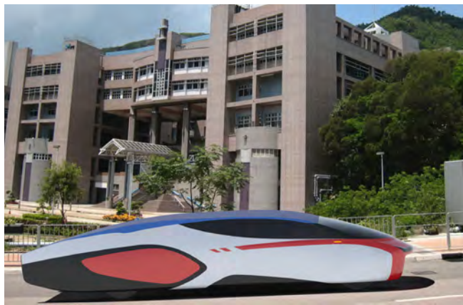
VTC SOLAR CAR TEAM SOPHIE 8X | REGION OF HONG KONG NO. 25 Since 2013, the team has competed in the World Solar Challenge five times, earning third place in the Cruiser Class in 2019. Their solar car reflects a commitment to zero-carbon energy and transportation, combining high-efficiency solar cells with an ultra-lightweight carbon fibre chassis. Notably, it is the first and only solar vehicle legally approved for public roads in Hong Kong — a milestone that highlights the team's engineering excellence. They're especially eager to connect with top global students, share innovations, and collaborate on the future of sustainable transport.
