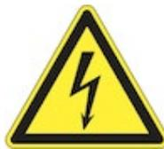
2.27.6 The high-voltage symbol must also be visible on any enclosure or barrier that can be accessed without using tools, if removing the enclosure or barrier exposes high-voltage parts.
